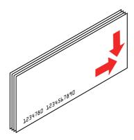
2 Insert documents straight with their faces (the side on which magnetic characters are printed) facing outside into the ASF, as shown in the picture below.
